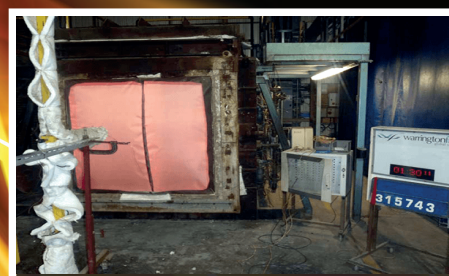
Phoenix after 90 minutes on a furnace at 1200° C
